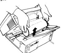
Pull up the top guide plate by loosening the blue screws.
